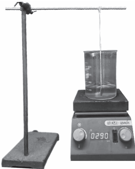
Figure 2. Experimental setup for the spontaneous deposition of ^{210}\text{Po} on a silver disc.
